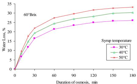
**Fig. 2** Variation in water loss with duration of osmosis at 60°Brix syrup concentration at three different syrup temperatures
