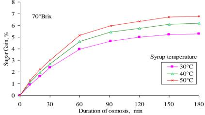
Fig. 6 Sugar gain with duration of osmosis at 70°Brix syrup concentration at three different syrup temperatures.
