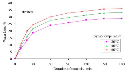
Fig. 3 Water loss with duration of osmosis at 70°Brix syrup concentration at three different syrup temperatures
