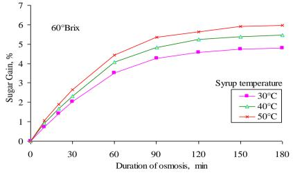
Fig.5 Sugar with duration of osmosis at 60°Brix syrup concentration at three different syrup temperatures.
